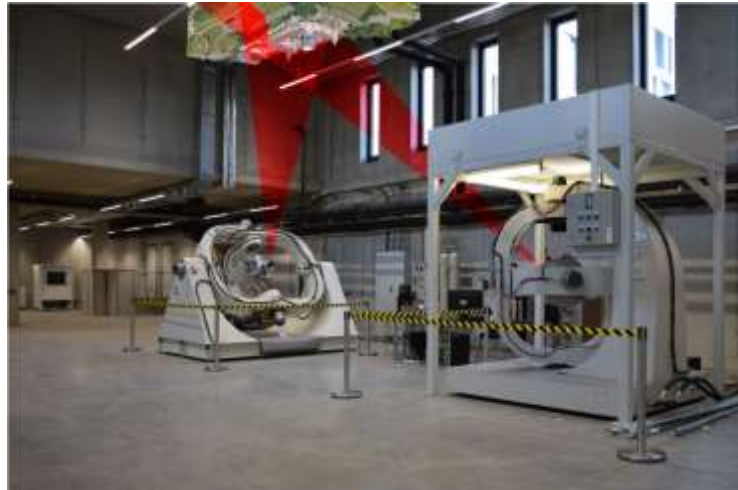
Fig.1: Two precision turntables providing a realistic attitude simulation background for testing the Earth observation characteristics for a satellite formation. The Earth surface model at the ceiling is moving to represent the orbit motion of the satellites.
