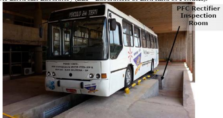
Figure 14: Inspection room for maintenance and access to the PFC rectifier.
