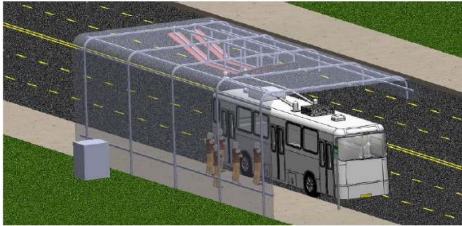
Figure 3: Feeding station built on the platform of boarding and landing passengers.
