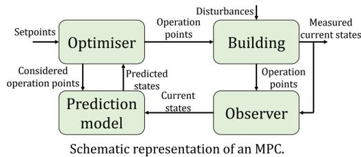
Schematic representation of an MPC.
