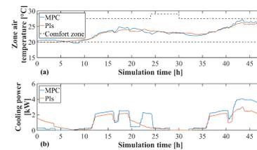
(a) Zone 10 air temperature and (b) rooftop unit cooling power consumption during the simulated time in summer.
