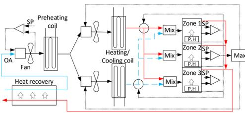
Representation of the HVAC system and control scheme.
